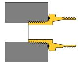
1. Screw the gland for Ex d or Ex e applications into the box or device For Ex d application at least 5 windings
