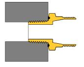
1. Screw the products for Ex d or Ex e applications into the box or device For Ex d applications at least 5 windings
